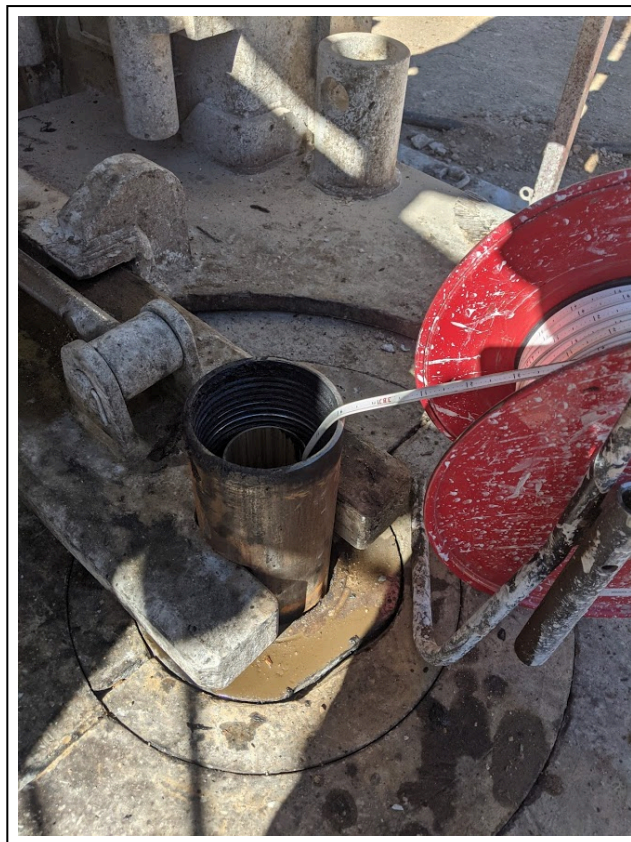
16. 2/6/2021: DBS&A field staff deploy a water sounder down the borehole to measure water recovery
