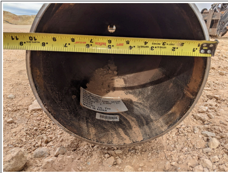
8. 2/10/2021: Surface conductor casing diameter measurement: 10 inches
